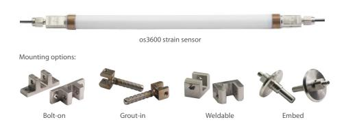
In side by side comparisons with foil strain gages, the os3600 is equally sensitive and accurate, while providing for greater strain range and 100 times more fatigue life. The os3600 strain gage is qualified for use in harsh environments and delivers the many advantages inherent to all FBG based sensors.
