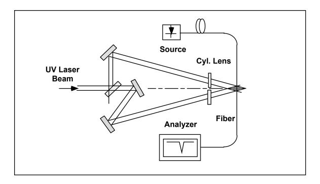
Figure 3.2 Two-beam interferometer for writing fiber Bragg gratings
