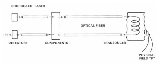
Figure 2.2: Basic elements of an optical fiber sensing system
