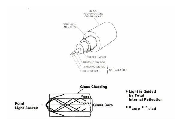
**Figure 2.1**: Schematic of an optical fiber. *II. Introduction to Optical Fiber Sensors*
