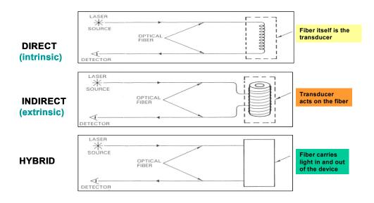
Figure 2.3: Classification of optical fiber sensors
