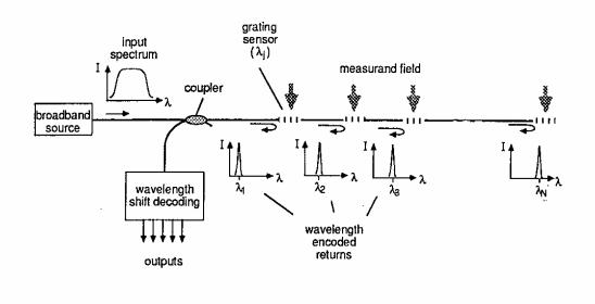
*Figure 3.4* Schematic representation of a WDM interrogation of a FBG array
