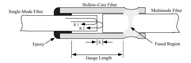
Figure 4.1 Aspect on an Extrinsic Fiber Fabry-Perot Interferometer sensor
