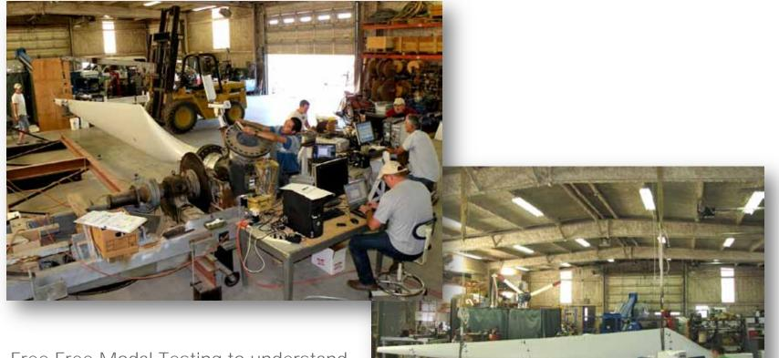
Free-Free Modal Testing to understand • SBlade structural dynamics.
