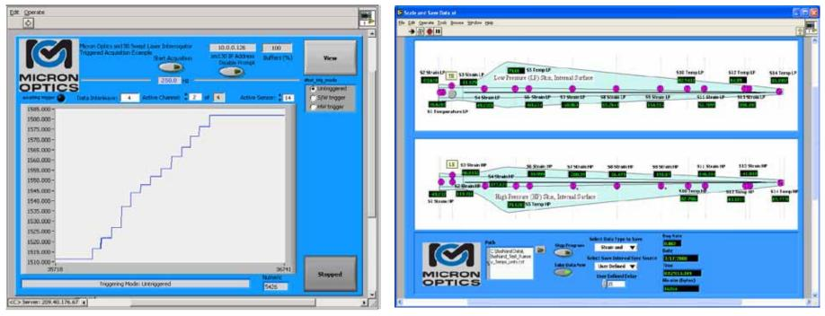
S This user interface provides for setting up the data acquisition parameters, selection of trigger source, and controlling the sm130. S This graphical user interface provides for visualization of the FBG sensor layout, scaling data, setting up of data file storage, and remote real-time monitoring.
