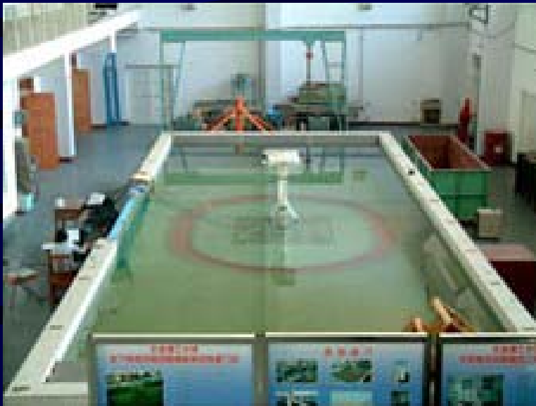
Fig.20. Model of the single post offshore platform immersed in water in the direction of east to west
