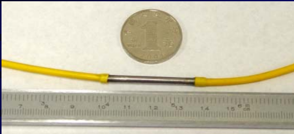
Picture of stainless steel tube-packaged FBG sensor.
