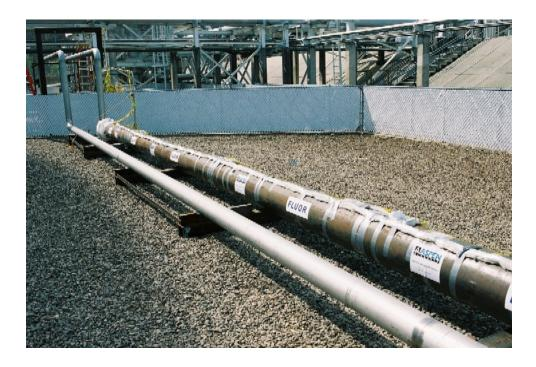
View of the cryogenic insulation test for a subsea pipeline configuration. Test was conducted in April 2004 under flowline LNG conditions during start-up, steady-state and shut-down. Twenty-two fiber-optic sensors were employed in the test.
