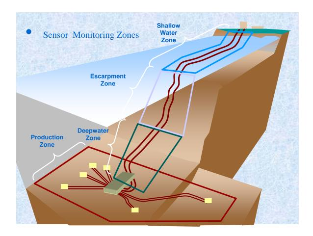
A typical application of fiber-optic sensors for a subsea pipeline solution would be as shown in the illustration below:
