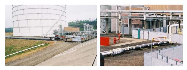
A recent test was conducted on a high-performance insulated pipe-in-pipe configuration using flowing LNG to simulate a subsea cryogenic insulated pipeline. Specialized fiber-optic heat-flux sensors were developed to monitor the thermal performance of the configuration.
